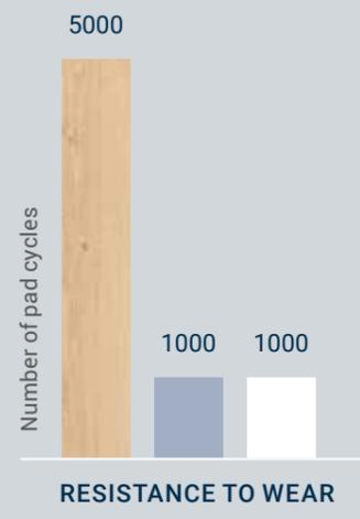
Wear resistance measurement (based on EN ISO 16094).
